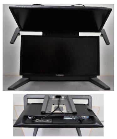
Plug the cables into the top monitor.
